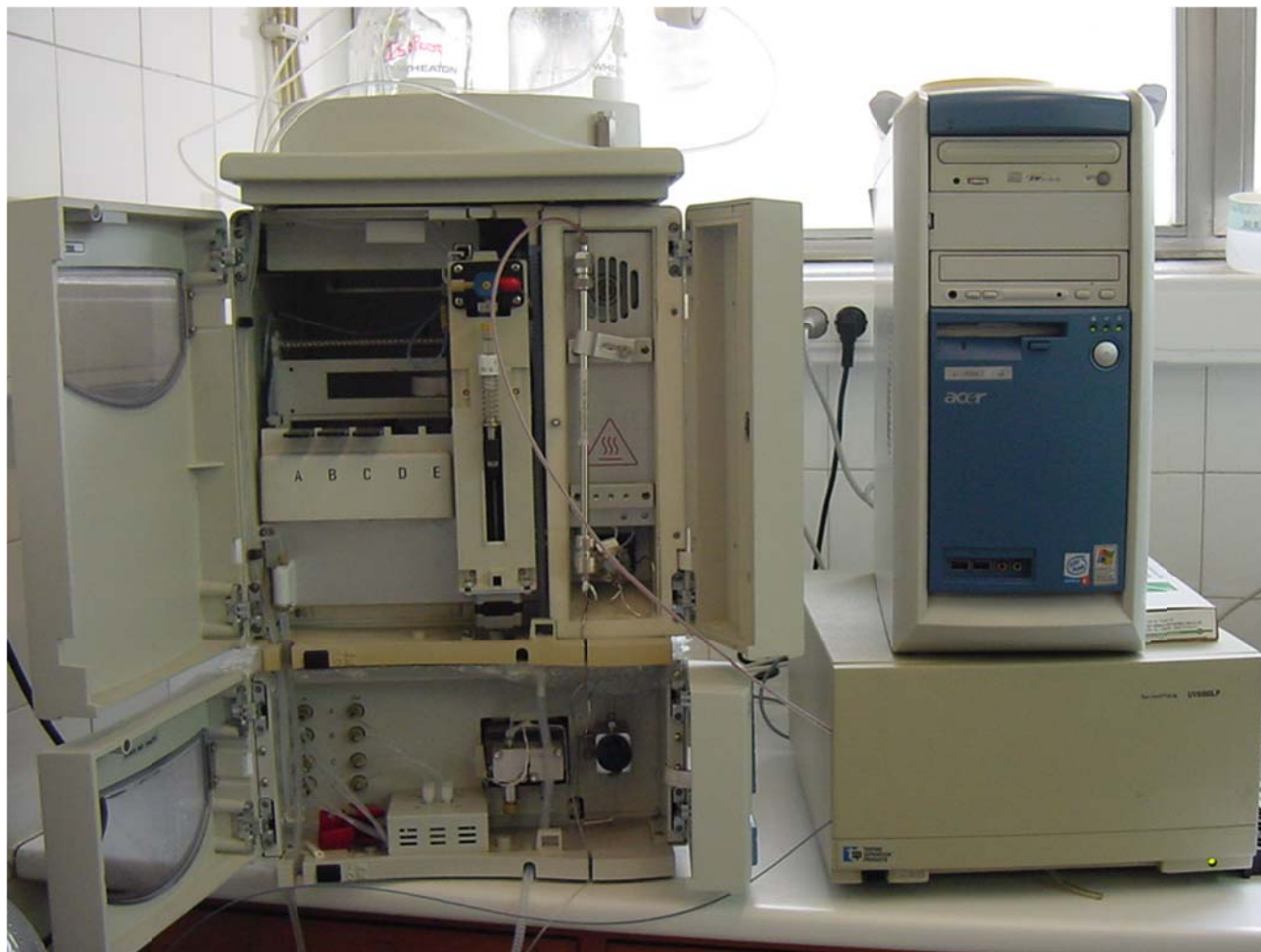
Figure SM 1.13.1 – Photo of HPLC equipment (Finnigan Surveyor (Thermo Electron Corporation, USA) equipped with an autosampler (AutoSampler Plus) and a diode array detector TSP UV6000LP (Thermo Separation Products, USA)).
