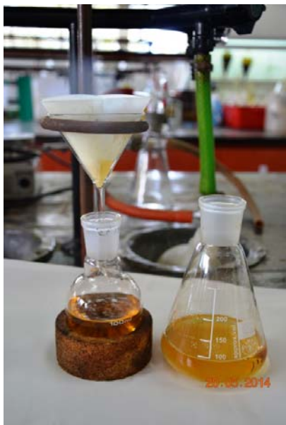
Fig.SM 1.8.5 Elimination of the drying agent.
