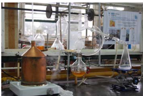
Figure SM 1.2.1: Steam distillation of orange oil.
