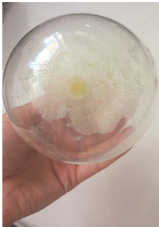
Figure SM 1.7.6. Crystals formed after recrystallization, (melting point 128-129° C).
