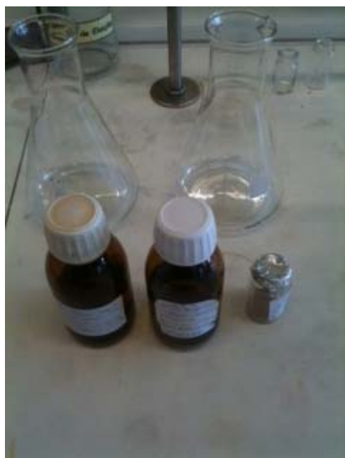
Fig. SM 1.1.3. Aqueous extracts A and B and recovered naphthalene
