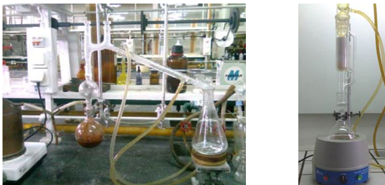
Figure 1.6.6. Photos of the steam distillation (left) soxhlet extraction (right) apparatus.
