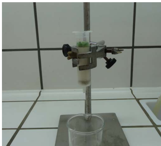
Figure SM 1.3.4 – Potato starch column chromatography immediately before elution (0 min).
