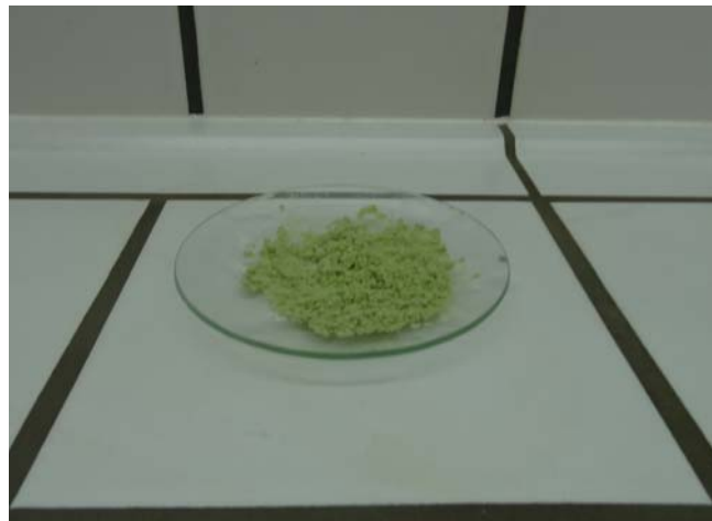
Figure SM 1.3.3 – Solid extract obtained by adsorption of the liquid extract (Fig SM 1.3.1c) on the surface of potato starch.
