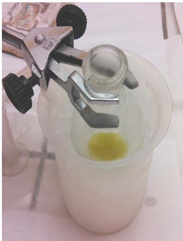
Figure SM 1.7.5. Piperine precipitation, using cold ether in an ice bath.
