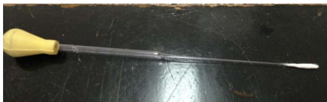
Fig. SM 1.5.3. Pipette adapted for acetone withdrawal.
