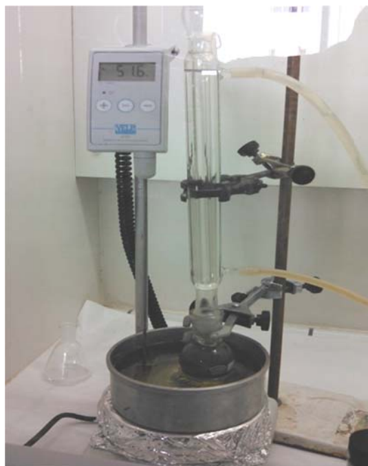
Figure SM 1.7.2. Reflux apparatus: water condenser attached to the top of the flask. Reflux temperature around 50°C for 20 minutes.
