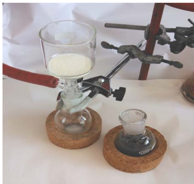
Figure SM 1.7.3. Vacuum filtration of pepper ground.
