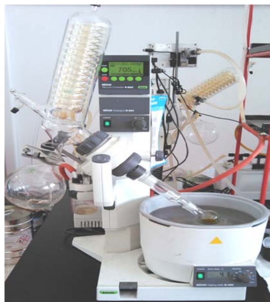
Figure SM 1.7.4. Solvent removal using a rotary evaporator.
